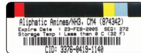
Figure 8-3: Chemcassette® Label with CID
